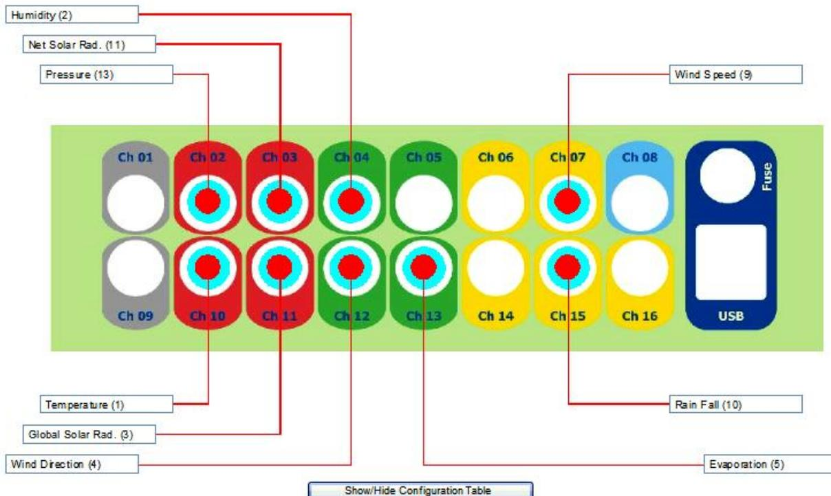
If using assembled Nesa or Ps2 cables, insert them one at a time with the machine off into the relative channel,
