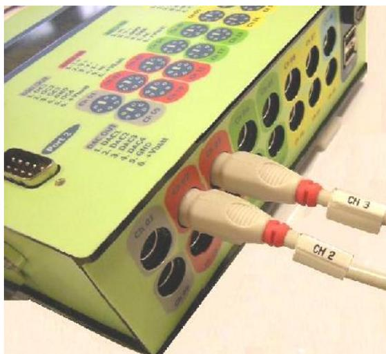
pushing the connector the whole way in so that the plastic of the connector is touching the TMF terminal. Pay close attention to the orientation of the connectors without forcing them and without damaging the connectors themselves.
